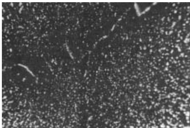
Figure 7.25. Inclusions of the second phase in the \text{ZrO}_2\text{-Y}_2\text{O}_3 10 mol.% + \text{N}_2\text{O}_3 0.5 mol% (electron microscopy) [40].
