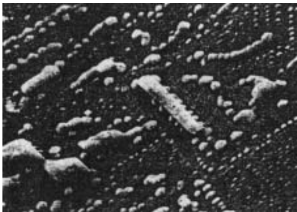
Figure 4.8. Electron micrograph of a \text{LaCrO}_3 ingot with an addition of 7 mol% of calcium chromite (for explanation see the text) [5].
