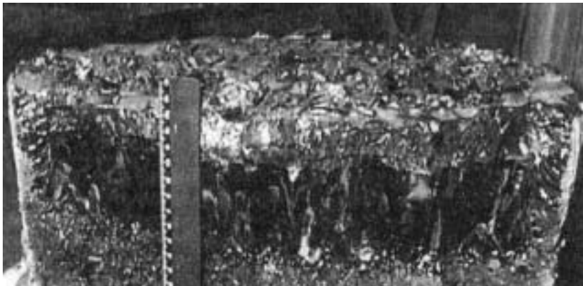
Figure 5.5. Block of crystals of cubic zirconia produced in a cold crucible.
